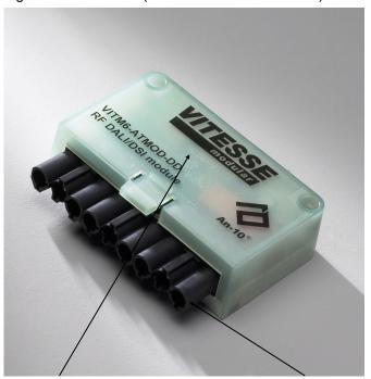
Clear casing which covers..... IR Receiver **Status LEDs**
