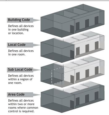
Note: for applications where there is only one channel of lighting being controlled in a room there is no need to select the channel number.
